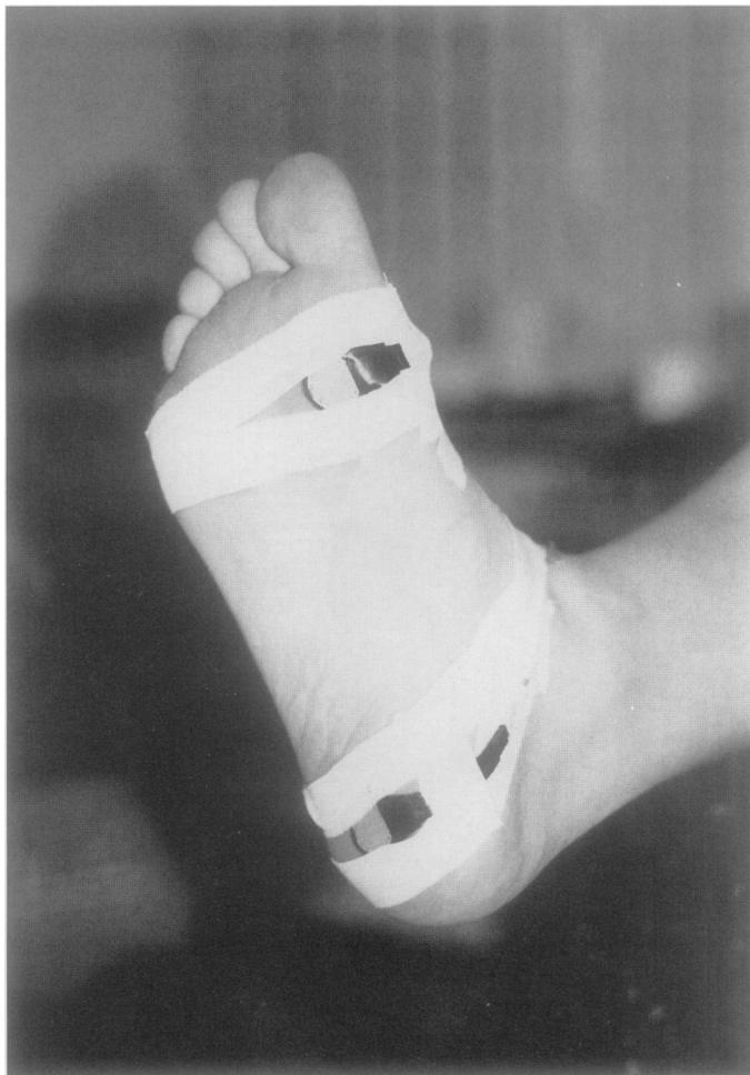
Figure 3. Two force-sensitive resistors (FSRs) secured to the head of the first metatarsal and heel mark ground and air phases of the functional activities.
