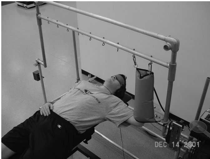
Figure 1. The proprioception testing device is a motor-driven jig used to test both position sense and kinesthesia. Subjects are fitted with a blindfold, headset containing white noise, and pneumatic sleeve to negate visual, audio, and tactile cues.
