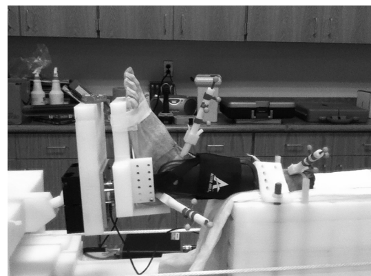
Fig. 1. Experimental setup with the foot in the ankle brace and the three markers attached to the calcaneus, talus and tibia.
