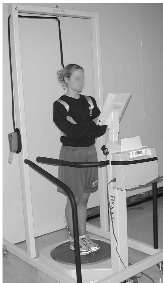
Fig. 2 Subject positioned on the Biodex Stability System (Biodex, Shirley, New York). The unstable platform is used to measure postural control under dynamic conditions.
